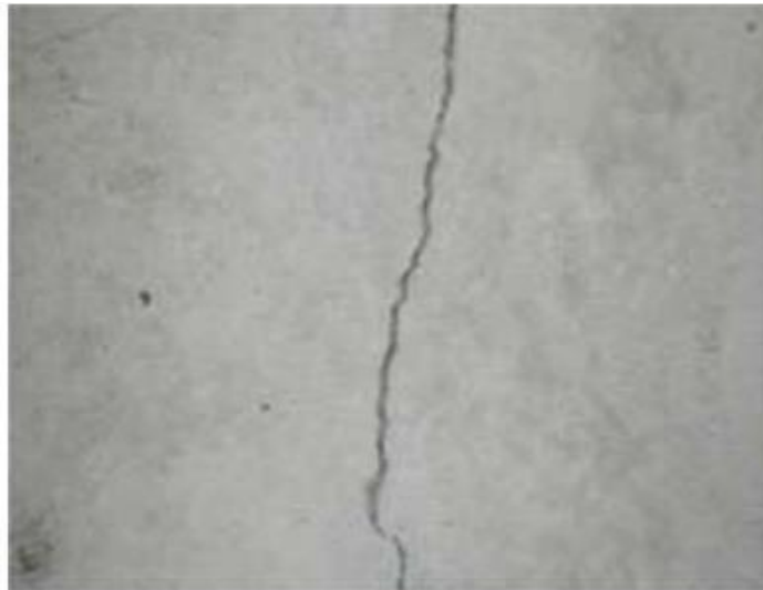
Plate.5 Reduction of thickness of crack size after healing
